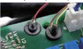
Example or probe with the double-sided tape
