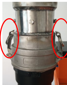
Cam lock adaptor in locked status.
